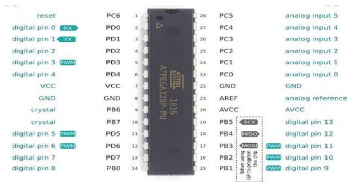
FIG.3.1.PIN DIAGRAM OF MICRO CONTROLLER
